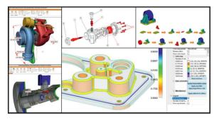
Explore and analyze your CAD data. Quickly navigate through assemblies, select parts, show or hide them, measure, cut or explode an assembly and much more.
